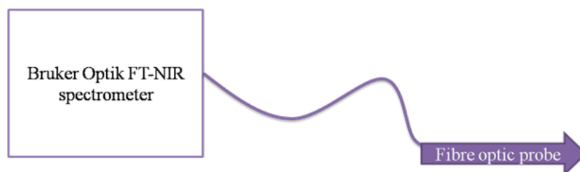
Fig. 12. Block diagram of Bruker-optik FT NIR-spectrometer for non invasive blood glucose monitoring device [36].
